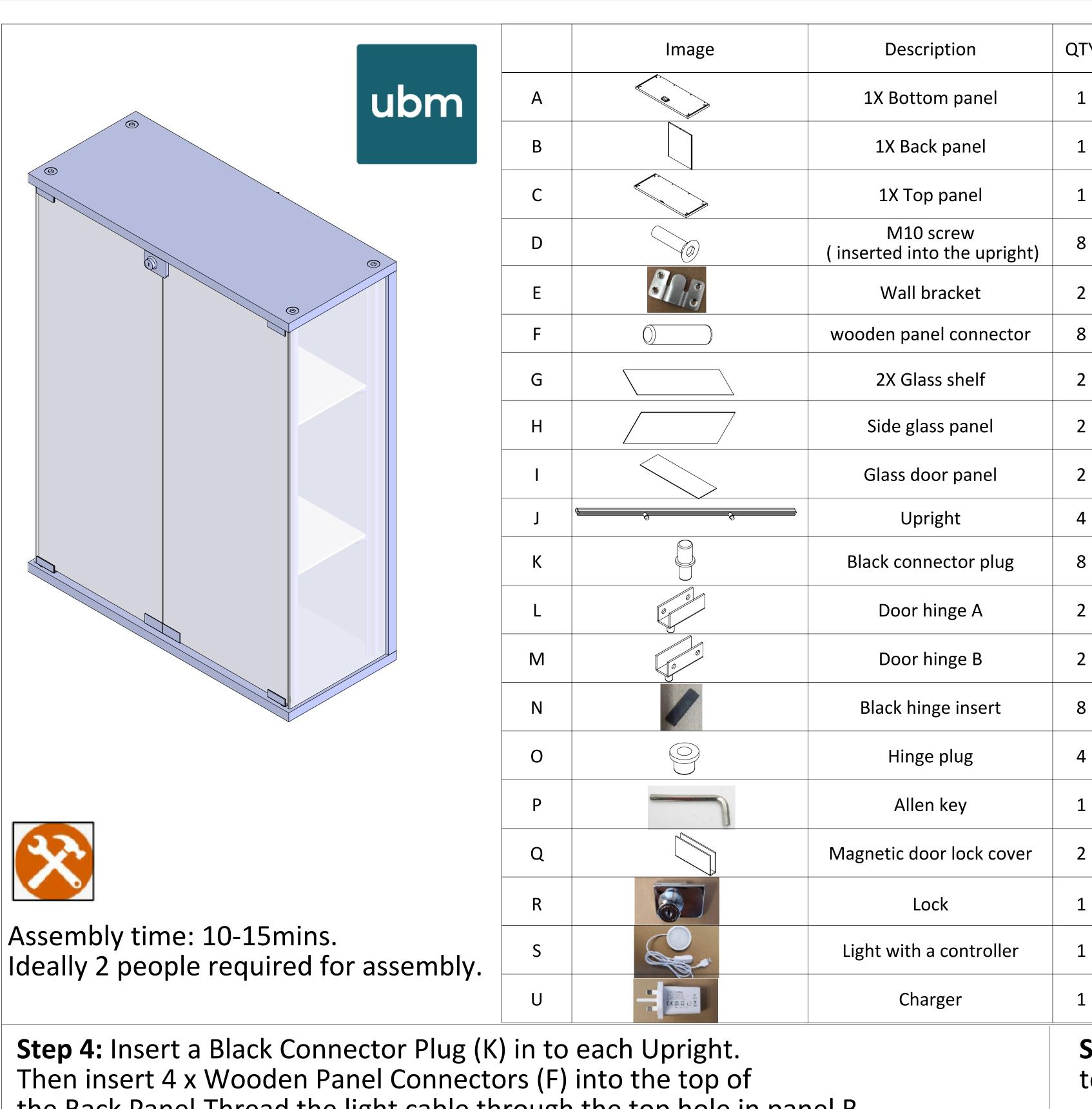
Step 1: Insert 4 x Black Connector Plugs (K) and 4 x Wooden Panel Connectors (F) into the Bottom Panel (A).
