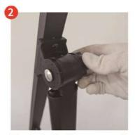
The central axis component is installed on the column, and the adjusting component is threaded through with a long screw. The screw nut is tightened by hand.
