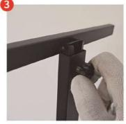
Insert the T-shaped bracket into the central axis and tighten the hand screws.
