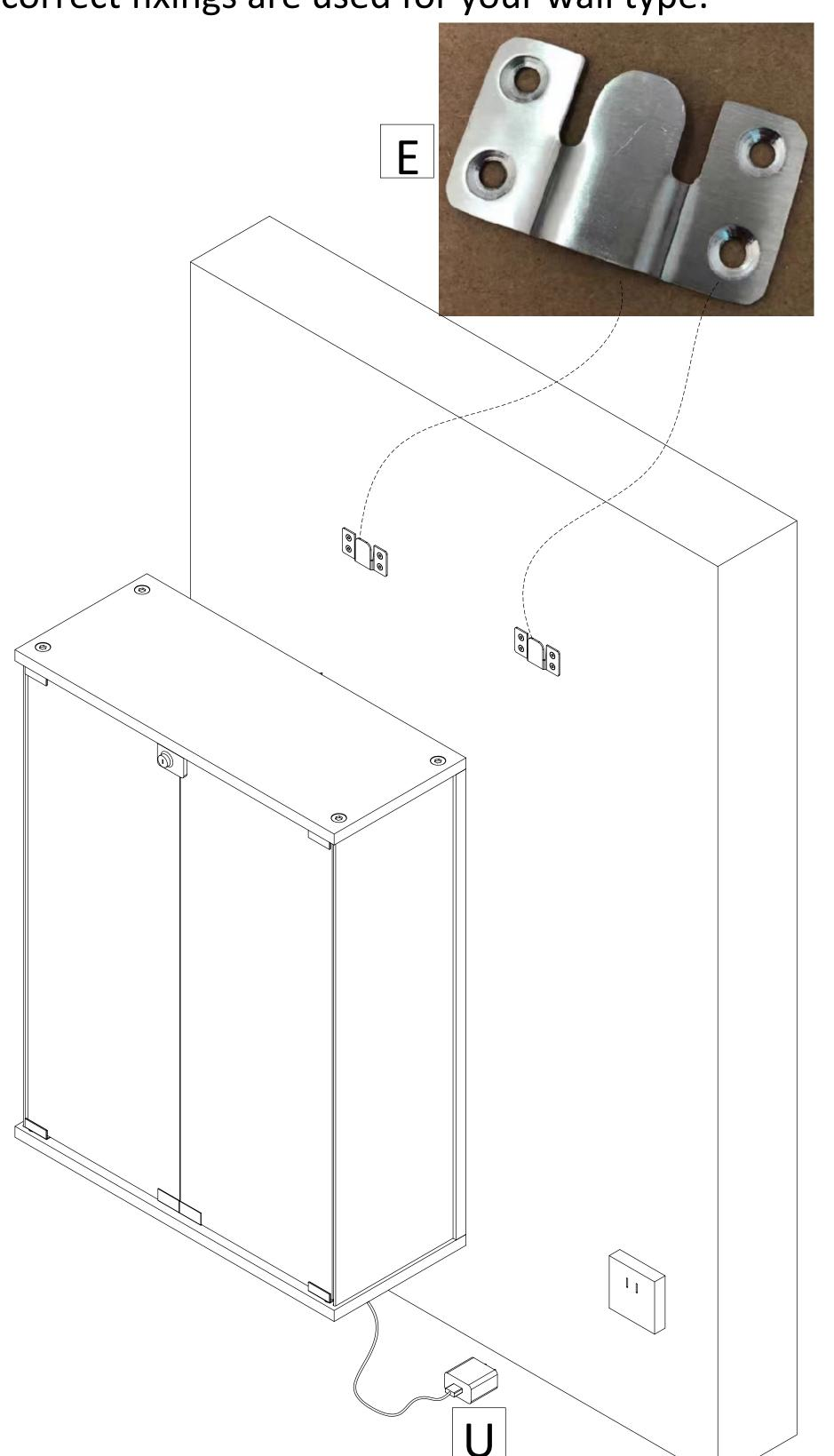
**Step 9:** Line up the Wall Brackets with the brackets on the Back Panel and slide the cabinet down.
