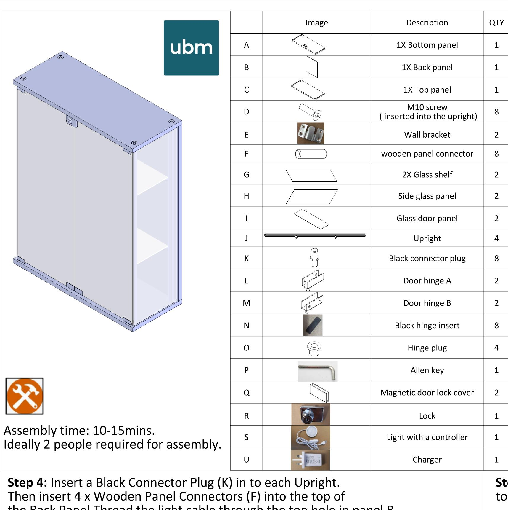
Step 2: Connect the Uprights (J) to the Bottom Panel with 4 x M10 Screws (D). Shelf supports are pre-inserted into the Uprights but can be adjusted if needed. To do so, loosen the Shelf Supports with a flat-head screwdriver and move up / down the upright channel. Tighten when in place. If you have purchased extra shelves, place the additional Shelf Supports into the Upright channels at this stage.
