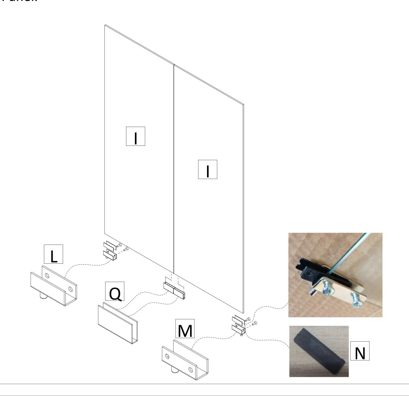
**Step 7:** Place the raised notches on the bottom Door Hinges into the Bottom Panel at each corner to begin to fit the Glass Door Panels in place. Place another Black Hinge Insert (N) into each remaining Door Hinge (L & M) – these will be for the top corners of each Glass Door Panel. Place one of the top Door Hinge notches into the hole in the corner of the Top Panel.
